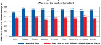
The ASTM D975 diesel fuel standard specifies a wear scar below 520  $\mu m$  in ASTM D6079 testing, while the Engine Manufacturers Association (EMA) specifies a wear scar below 460 um. Testing reveals AMSOIL Diesel Injector Clean provides significant lubricity improvement in diesel fuels found across the U.S., delivering improved wear protection
