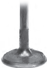
Intake Valve after P.i. Treatment
