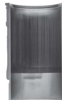
Severely Scuffed Liner
